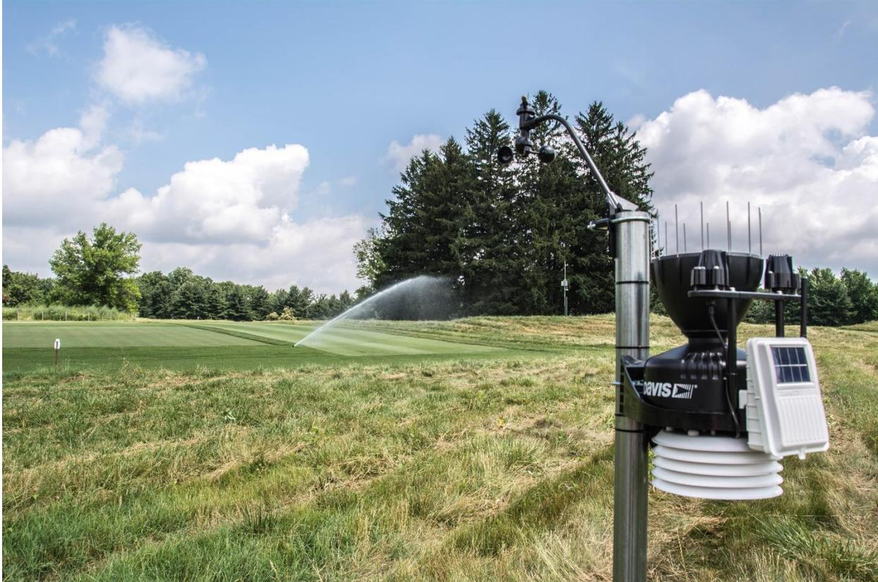
*Figure 12. On-site weather stations access weather information and ET rates to determine site-specific water needs. Photo credit: Mark Jones.*
