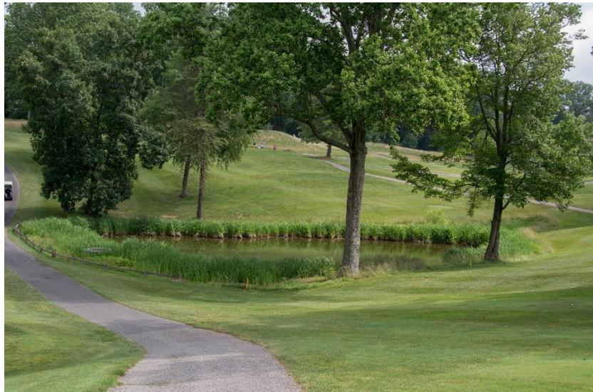
*Figure 15. Many BMPs to manage stormwater prolong the water detention process as long as practical, as in this detention pond at Baltimore Country Club. Photo credit: Mark Jones.*
